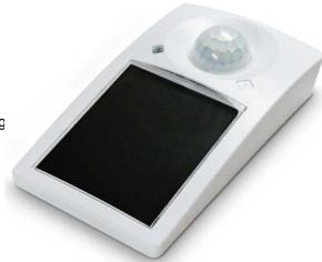
**Self Powered sensor** uses a photocell to collect and store energy from ambient indoor light for operation in complete darkness for up to 4 days. An option battery may be installed for operation in rooms that may be dark for longer than 4 days at a time.
