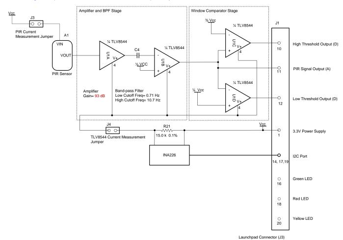
Figure 3. BOOSTXL TLV8544PIR BoosterPack Conceptual Diagram
