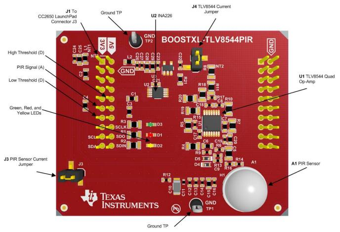
Note: A – Analog signal, D – Digital signal, Bold Text – BOOSTXL-TLV8544PIR component reference designator **Figure 4. BOOSTXL-TLV8544PIR BoosterPackBoard (Top View)**
