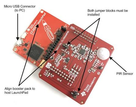
Note that both jumper blocks must be installed for proper operation.
