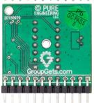
The C12880MA Breakout Board by GroupGets is a simple Arduino compatible breakout board for the Hamamatsu C12880MA MEMs micro-spectrometer. The C12880MA Spectrometer is used to detect wavelengths of light and their intensities. This sensor is the successor to the C12666MA spectrometer and offers a greater spectral range and resolution.
