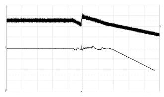
Input Voltage transient. Hold-up sequence with PIM4710 at: TP1= +25°C, VI = 53 V, I\_0 = 96.2 A resistive load.
