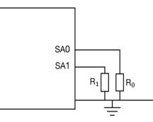
Schematic of connection of address resistors
