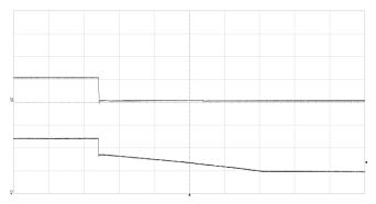
Shut-down enabled by disconnecting V<sub>I</sub> at:  $T_{P1}$ = +25°C, V<sub>I</sub> = 53 V,  $I_0$  = 96.2 A resistive load.
