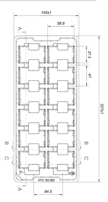
JEDEC standard tray for 2x6 = 12 products. All dimensions in mm Tolerances: X.x ±0.26 [0.01], X.xx ±0.13 [0.005] Note: pick up positions refer to center of pocket. See mechanical drawing for exact location on product.
