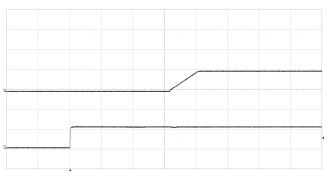
Start-up enabled by connecting V<sub>I</sub> at:  $T_{P1}$  = +25°C, V<sub>I</sub> = 53 V,  $I_{O}$  = 96.2 A resistive load.
