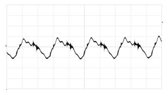
$\begin{array}{l} Output \ voltage \ ripple \ at: \\ T_{P1} = +25^{\circ}C, \ V_{I} = 53 \ V, \\ I_{O} = 96.2 \ A \ resistive \ load. \end{array}$
