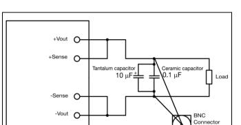
Output ripple and noise test setup
