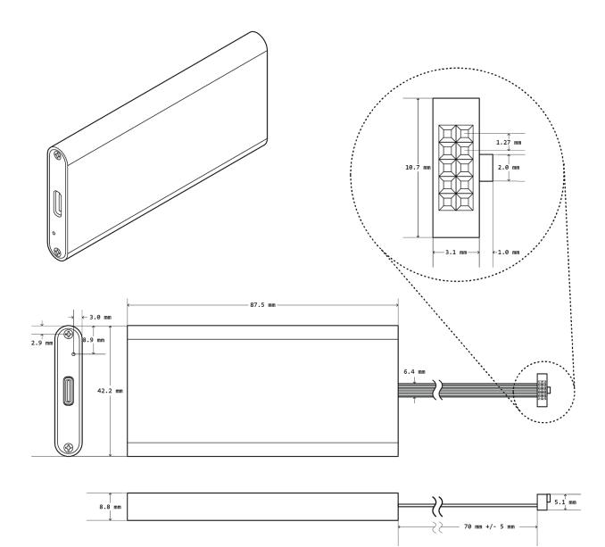
Binho Multi-Protocol USB Host Adapter Dimensioned Drawing
