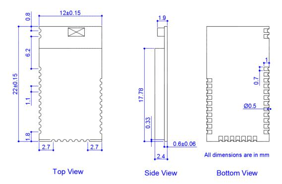
Figure 3: Mechanical Drawing
