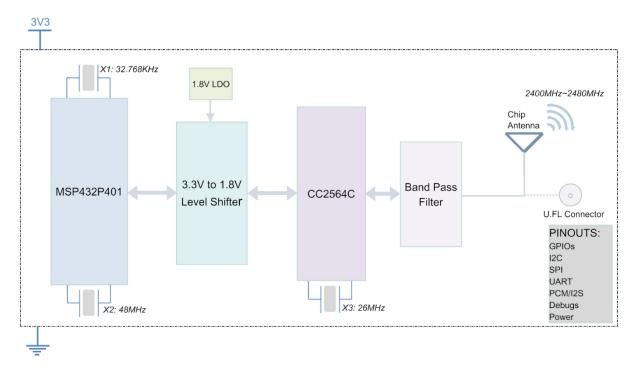
Figure 1: BDM209A Module Block Diagram
