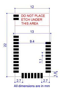
**Figure 4: Module Footprint Top View**
