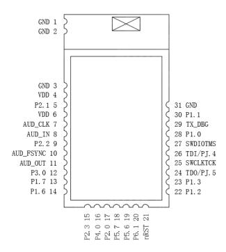
Figure 2: Pinout Diagram Top View
