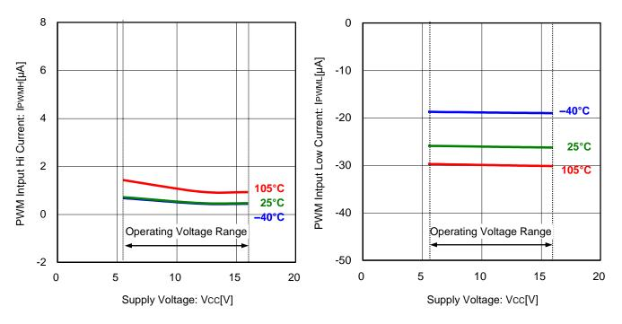
Figure 15. PWM Input Hi Current vs Supply Voltage
