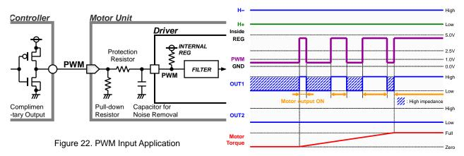
Figure 23. PWM Input Operation Timing Chart
