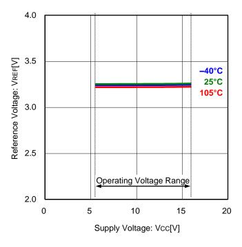
Figure 17. Reference Voltage vs Supply Voltage (IREF=-1mA)
