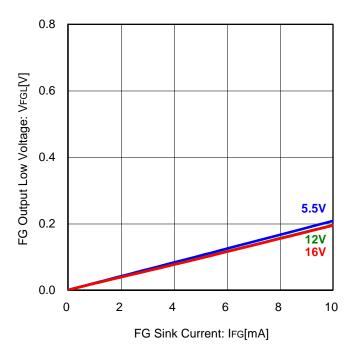
Figure 13. FG Output Voltage vs FG Sink Current (Ta=25°C)
