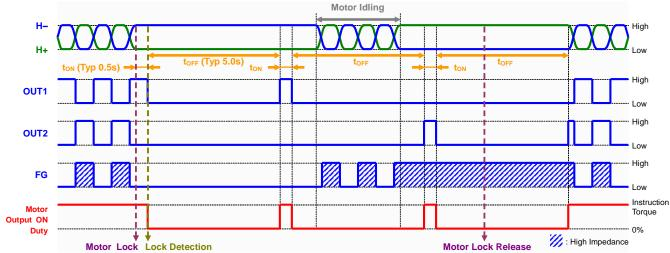
Figure 43. Lock Protection (Incorporated Counter System) Timing Chart
