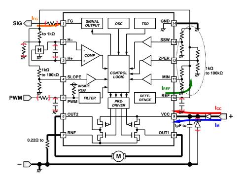
Figure 55. Current Pathway of IC
