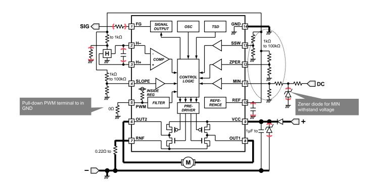
Figure 21. DC Voltage Input Application
