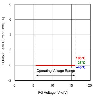
Figure 14. FG Output Leak Current vs FG Voltage
