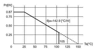
(Note)Reduce Reduce by 7.0mW/°C when operating over Ta=25°C (Mounted on 70.0mm x 70.0mm x 1.6mm glass epoxy board)
