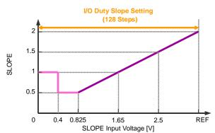
Figure 27. Adjust of Slope of I/O Duty
