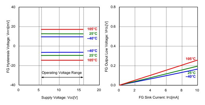
Figure 11. FG Hysteresis Voltage vs Supply Voltage
