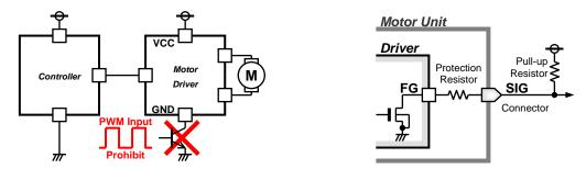
Figure 53. GND Line PWM Switching Prohibited
