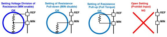
Figure 26. MIN Terminal Setting
