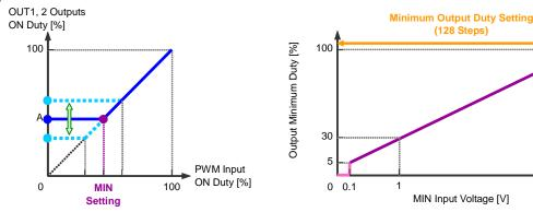
Figure 24. Setting of Minimum Output Duty
