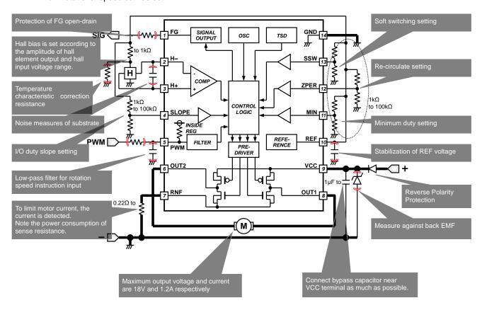
Figure 20. PWM Input Application
