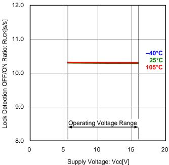
Figure 9. Lock Detection OFF Time vs Supply Voltage
