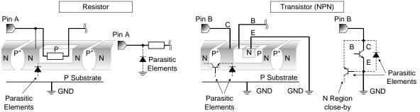
Figure 58. Example of monolithic IC structure
