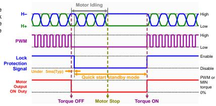
Figure 44. Quick Start Timing Chart (PWM Input Application)
