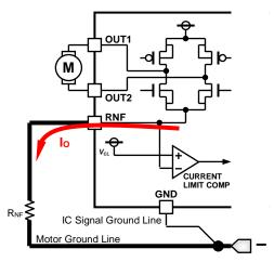
Figure 42. Setting of current limit and grout lines
