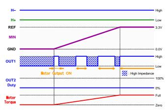
Figure 31. DC Input Operation Timing Chart
