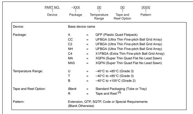
Note 1: Tape and Reel identifier only appears in the catalog part number description. This identifier is used for ordering purposes and is not printed on the device package. See "Orderable Part Numbers" below or check with your Microchip Sales Office for package availability with the Tape and Reel option.
