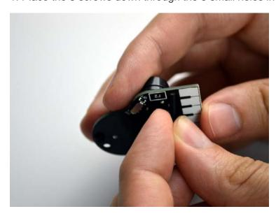
2. Place 3 nuts onto the 3 screws and tighten them down against the circuit board. These create the "piano legs".
