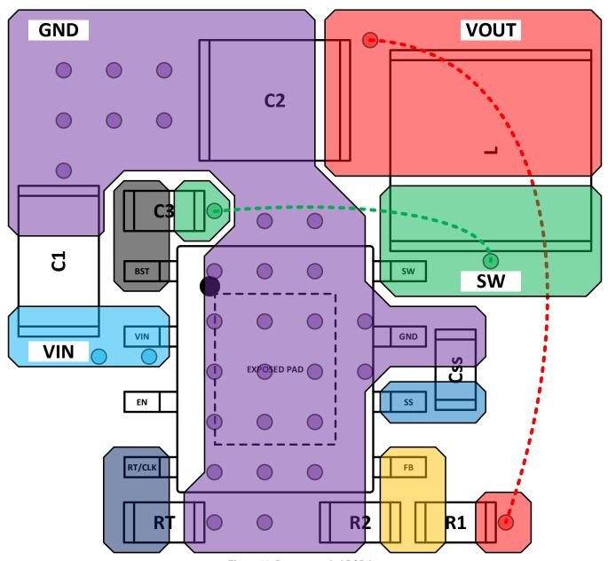
Figure 26. Recommended PCB Layout
