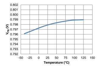
Figure 8. Feedback Voltage vs. Temperature
