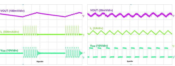
Figure 14. Output Voltage Ripple, IOUT = 50mA
