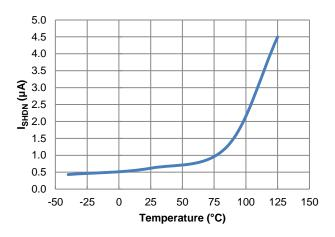
Figure 10. IQ vs. Temperature
