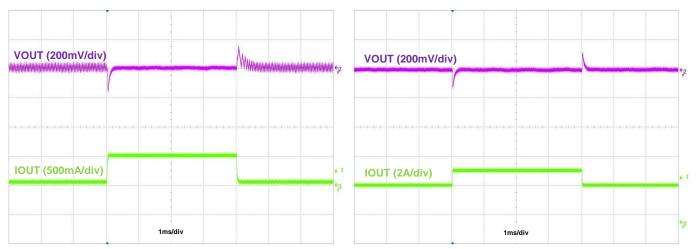
Figure 16. Load Transient, IOUT = 50mA to 500mA to 50mA
