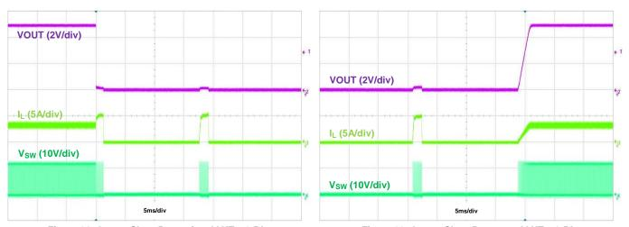
Figure 21. Output Short Protection, IOUT = 3.5A
