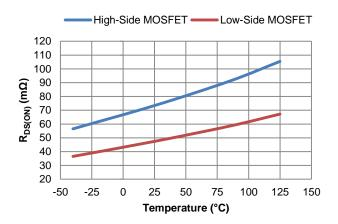
Figure 9. Power MOSFET R<sub>DS(ON)</sub> vs. Temperature
