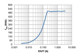
Figure 13. f<sub>sw</sub> vs. Load
