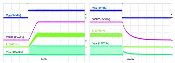
Figure 19. Startup Using EN, IOUT = 3.5A
