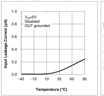
Input Leakage Current vs. Temperature
