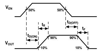
Figure 1. Voltage Waveforms: AP22804B/AP22814B (Active Low, Left), AP22804A/AP22814A (Active High, Right)
