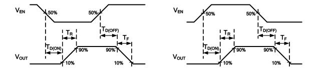
Figure 1. Voltage Waveforms: AP2182A (left), AP2192A (right)
