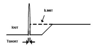
Figure 2. Response Time to Short-Circuit Waveform
