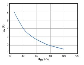
Figure 30. Current Limit vs RLIM
