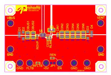
Figure 31. Evaluation Board Layout
