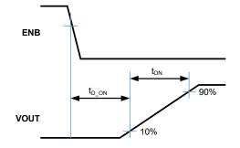
Figure 1. Turn-on Delay and Turn-on Time
