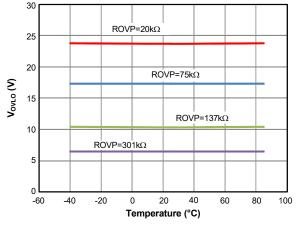
Figure 29. VBUS OVP vs. Temperature
