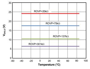
Figure 28. VINT OVP vs. Temperature
