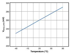
Figure 27. UVLO Hysteresis Voltage (VBUS) vs. Temperature
