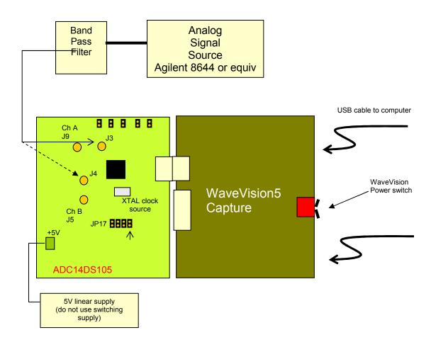
Figure 2. Test Set up
