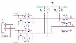
Figure 2: DC Coupled Input Configuration
