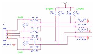
Figure 3: AC Coupled Input Configuration
