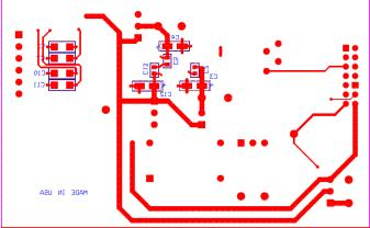
Figure 13: ADC122S706 Evaluation Board: Bottom Layer
