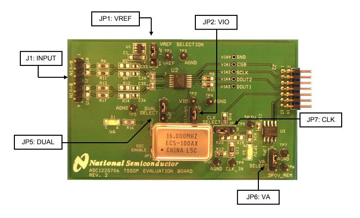
Figure 1 Component and Test Point Locations
