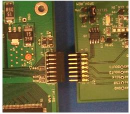
Figure 4: WV4 to ADC122S706 Connection
