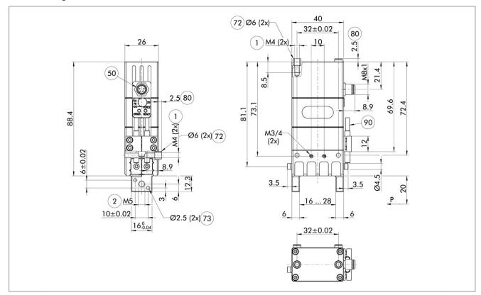
The drawing shows the basic version of the gripper with open jaws, without dimensional consideration of the options described below.
