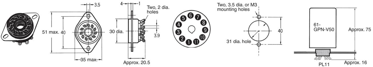
**Important:** Install the Water Leak Detector socket with the keyway facing down.
