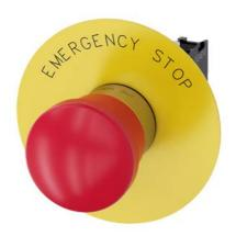
EMERGENCY STOP mushroom pushbutton, 22 mm, round, metal, shiny, red, 40 mm, positive latching, acc. to EN ISO 13850, pull-to-unlatch mechanism, with yellow backing plate, inscription: EMERGENCY STOP, with holder, 1 NC, screw terminal
