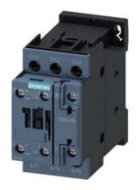
power contactor, AC-3 25 A, 11 kW / 400 V 1 NO + 1 NC, 110 V AC, 50 Hz, 120 V, 60 Hz, 3-pole, Size S0, screw terminal
