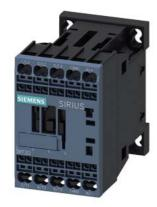
Power contactor, AC-3 9 A, 4 kW / 400 V 1 NO, 24 V DC 3-pole, Size S00 Spring-type terminal
