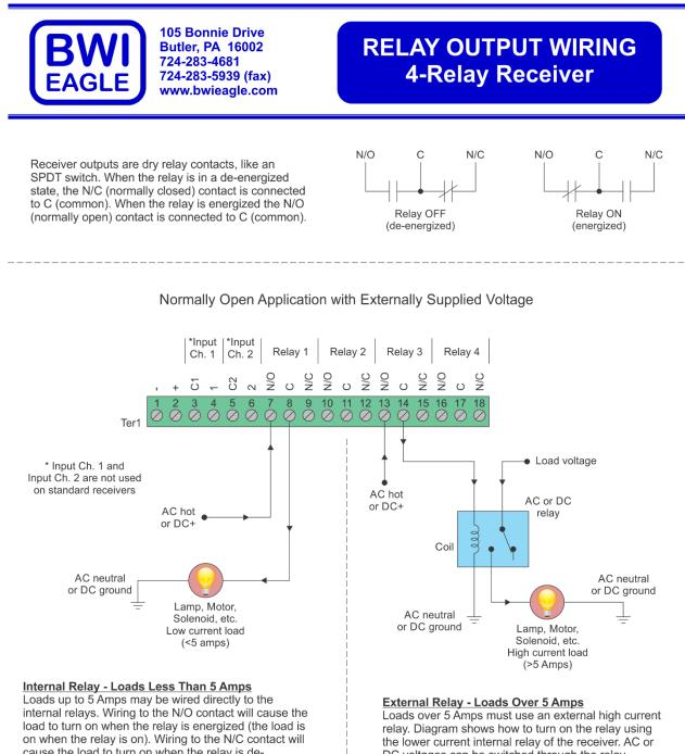
on when the relay is on). Wiring to the N/C contact wil cause the load to turn on when the relay is deenergized (the load is on when the relay is off). AC or DC voltages can be switched through the relay. the lower current internal relay of the receiver. AC or DC voltages can be switched through the relay. Note: A protection diode for DC coils or an MOV for AC coils is recommended to reduce inductive EMI noise.
