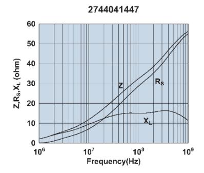
Impedance, reactance, and resistance vs. frequency.
