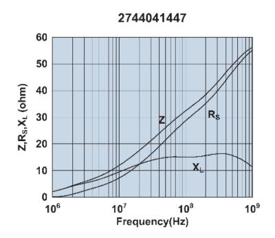
Impedance, reactance, and resistance vs. frequency.
