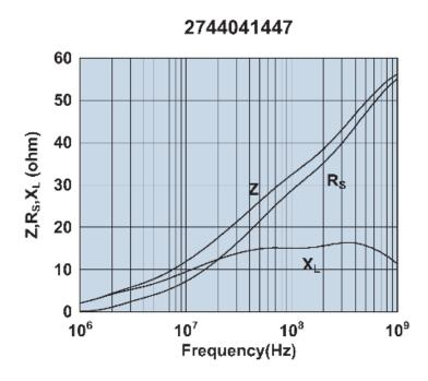
Impedance, reactance, and resistance vs. frequency.
