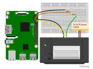
Printer RX (yellow) to Pi serial TXD. Printer ground (black wire next to yellow) to Pi GND. Printer TX to one side of a 2.2KΩ resistor.
