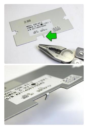
On the back plate, there's a small metal "finger" between the serial and power sockets. Using pliers, this can be bent back to provide an exit route for the DTR wire.
