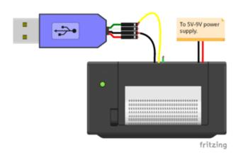
USB TX to printer RX USB Ground to printer Ground
