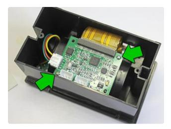
Take the back plate off, then remove the two (or sometimes four) Phillips screws holding the circuit board in place.
