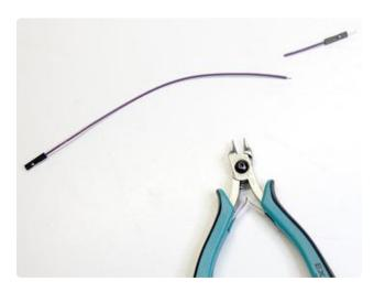
Cut an end off a female jumper wire and strip & tin the end.
