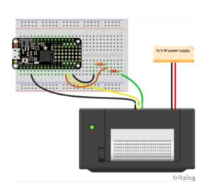
Printer power positive (red wire) to 5-9V DC power supply positive. Printer power ground (black wire next to red) to power supply negative / ground. Printer RX (yellow) to board serial TX. Printer ground (black wire next to yellow) to board ground / GND. Printer TX to one side of a 2.2K $\Omega$  resistor. One side of a 3.3K $\Omega$  resistor to the opposite side of the 2.2K $\Omega$  resistor. Other side of the 3.3K $\Omega$  resistor to board ground / GND.
