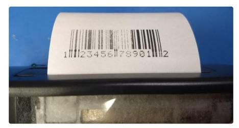
The first parameter to print\_barcode is a string that defines the barcode value (this varies depending on the type of barcode, a UPC A code is 13 digits). The second parameter is the type of the barcode, which again is dependent on the printer firmware. Typical values you might use include:
