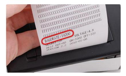
If no baud rate is shown, or your printer has no self-test page feature, try using 9600 as the default.
