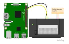
Pi GND to printer Ground (black wire) Pi TXD to printer RX (yellow wire)
