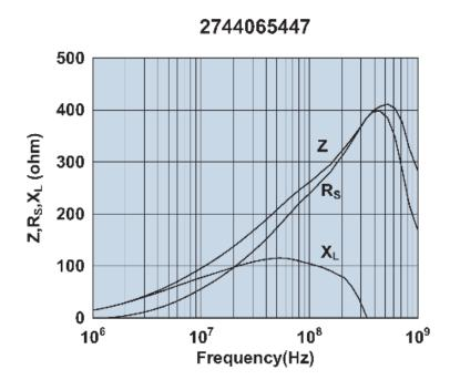
Impedance, reactance, and resistance vs. frequency.
