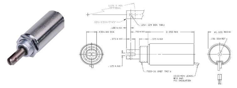
Solenoid shown energized with plunger fully seated Supplied with hex nut shipped loose Spring kits available (consult factory)
