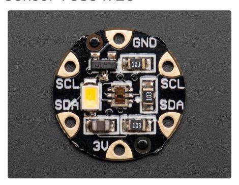
You can detect the color of an object with the TCS34725 color sensor. The onboard LED shines onto the object, reflecting light into the sensor for an accurate color reading, great for matching your accessories to your outfit like in the <a href="Chameleon">Chameleon</a> Scarf (https://adafru.it/dNd) or FLORAbrella (https://adafru.it/dNe).
