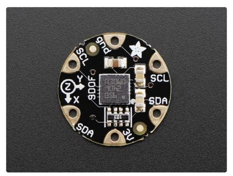
If you need even more motion data, the 9 degrees of freedom sensor is the new LSM9DSO which has a gyroscope as well, all together great for sensing orientation and heading in 3D space.
