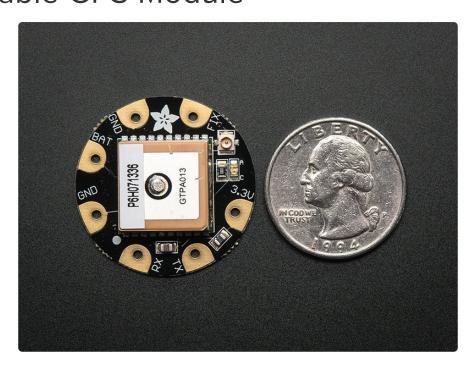
This module is the best way to add a GPS to your wearable project. Installed on the PCB is the latest of our Ultimate GPS modules, a small, super-thin, low power GPS module with built in data-logging capability! This module's easy to use, but extremely powerful. It's does not use i2c like the other sensors, but rather communicated over serial to FLORA. Use it for a GPS Jacket (https://adafru.it/dNi) of GPS logging dog harness (https://adafru.it/dNj).
