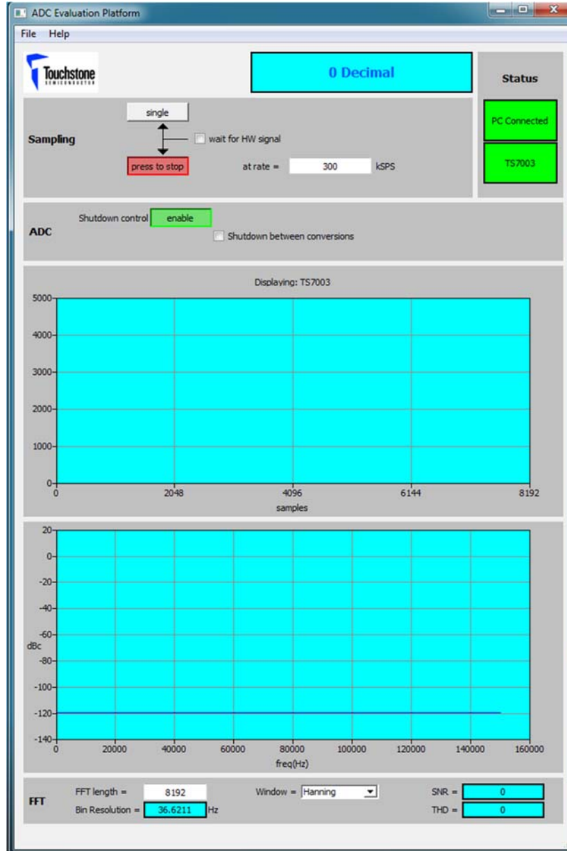
Figure 4. TS7003 Shutdown Control Enabled
