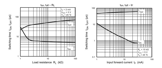
Note: The above characteristics curves are presented for reference only and not guaranteed by production test, unless otherwise specified.
