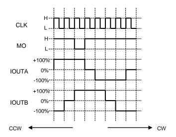
Waveform of MO output: State of pull-up.
