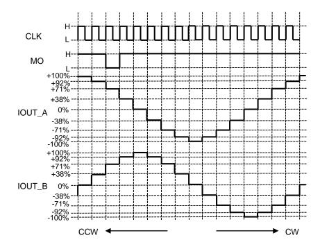
Waveform of MO output: State of pull-up.
