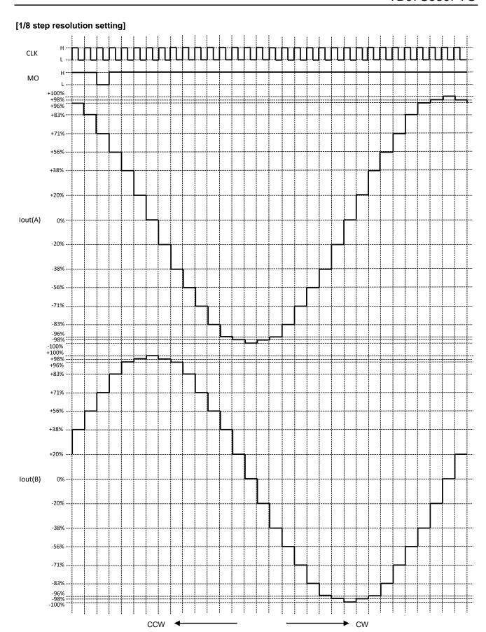
Waveform of MO output: State of pull-up.
