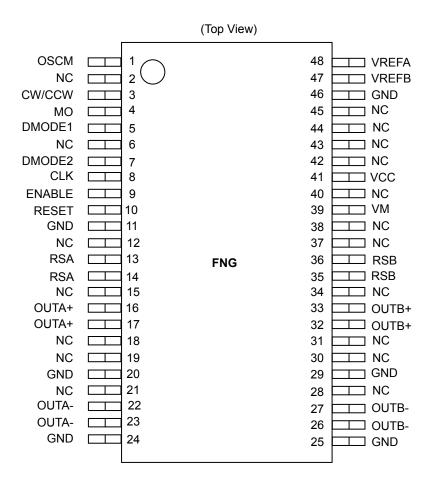
Please mount the exposed pad of the HTSSOP package to the GND area of the PCB.
