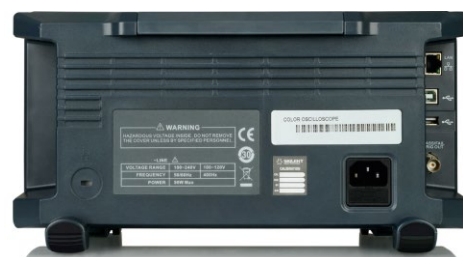
Back panel of T3DSO1104, T3DSO1202A, T3DSO1204, T3DSO1302A
