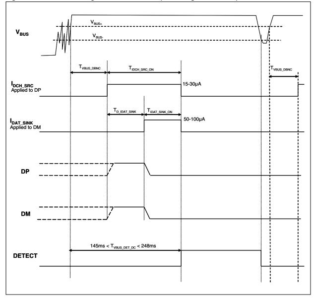
Figure 5. Dedicated charger detection method (with charger connected)
