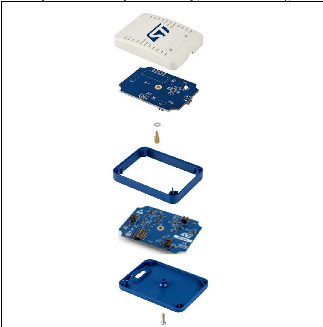
Figure 16. Closed casing for STM32 debug (STDC14 connector only)
