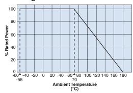
For resistors operated at an ambient temperature of 70°C or above, a power rating shall be derated in accordance with the above derating curve.
