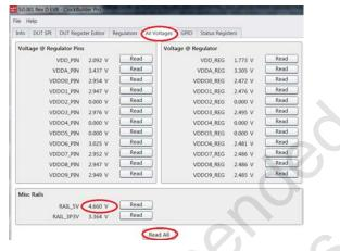
Figure 5.2. EVB GUI - Power Supply Check
