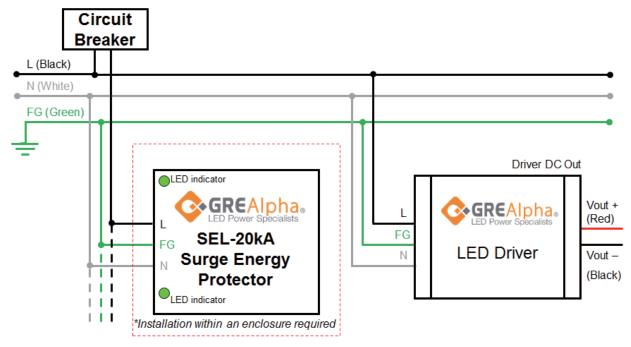
N.B. During normal operation, both LED indicators will light on. If any one or both LED indicator is off, replacement is needed.
