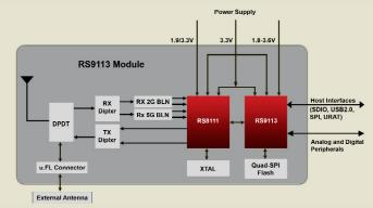
RS9113 Module Block Diagram with integrated antenna
