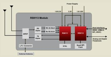
RS9113 Module Block Diagram without integrated antenna
