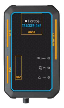
As the GNSS antenna faces the top of the case, you also want the top of the case facing the sky to the greatest extent possible. You will likely be be unable to get a GNSS lock with the top facing down.
