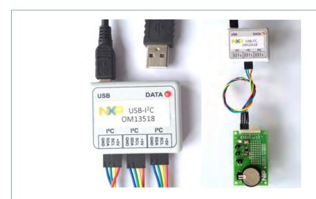
Fig 5. A) Dongle OM13518, B) connected to an evaluation board
