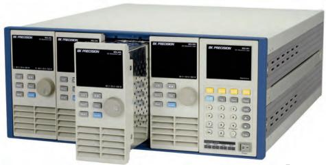
The MDL Series is a multi-channel modular programmable electronic load system. Six different modules of programmable DC loads ranging in power from 200 W to 600 W provide users the flexibility to test a wide range of power sources from multi-output AC/DC power supplies to batteries, fuel cells, and photovoltaic arrays.
