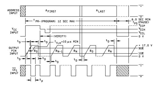
NOTE: All other waveforms characteristics shall be as specified in table IVC.
