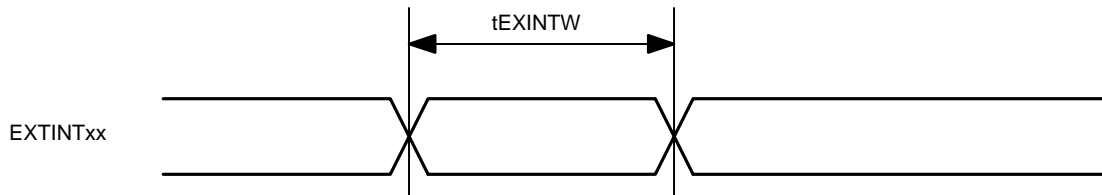
Figure 8. AC Characteristic – External Interrupt
