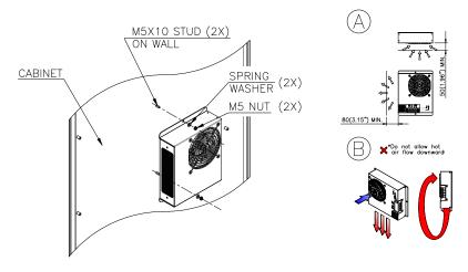
\*Note A. Mimum gap for air inlet and exit is required to avoid the damage caused from blocked
