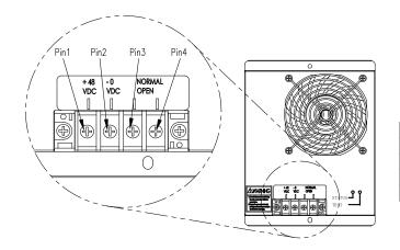
Dry contact : (Contact max. rating: <u>60VDC/50mA</u>)
