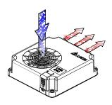
\*Note A. Mimum gap for air inlet and exit is required to avoid the damage caused from blocked air passage
