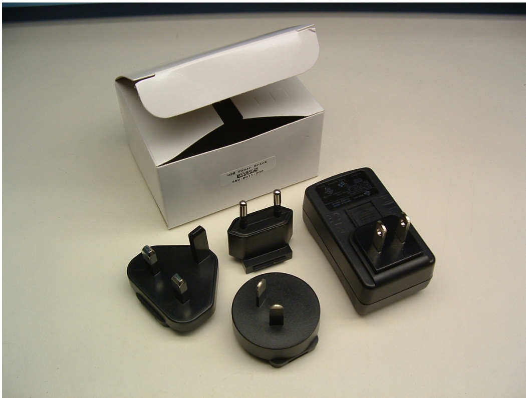
Figure 3-5. USB power supply with interchangeable AC adapters
