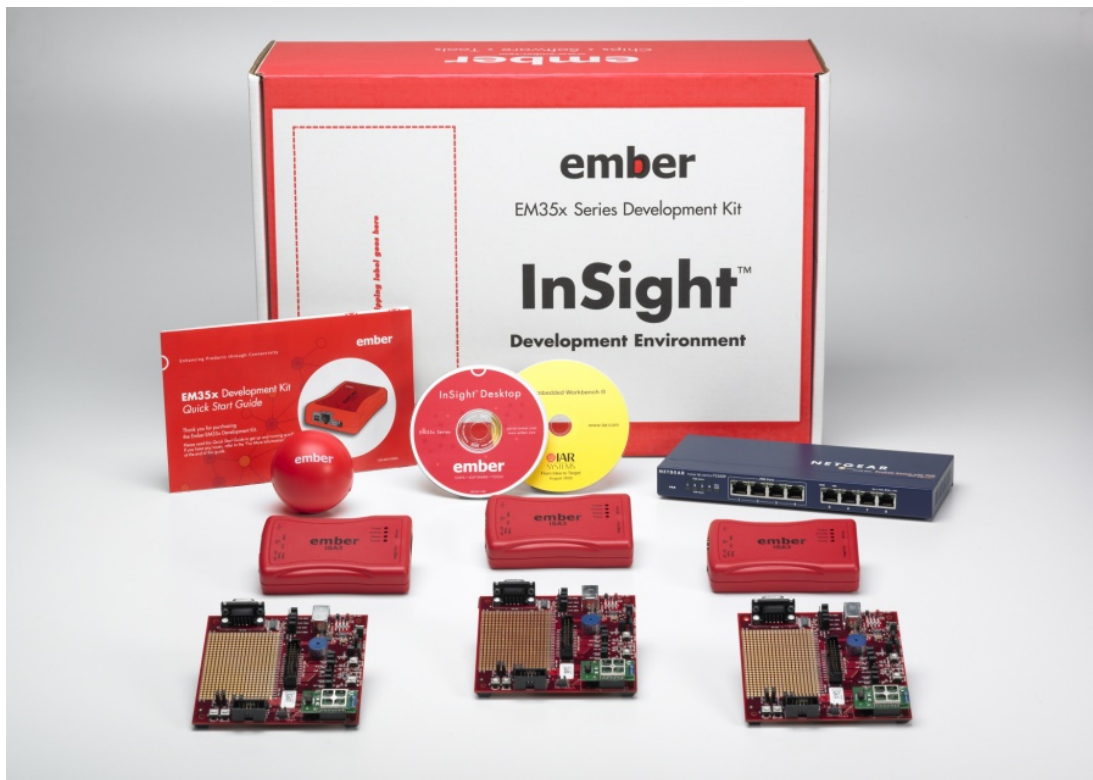
Figure 3-1. EM35x Series Development Kit
