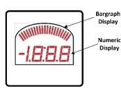
**Bar-graph Display:** The 21 segment bar-graph display responds quickly and smoothly like an analog meter movement to aid in reading rapidly changing measurements.
