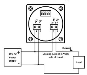
It is also possible to use the meter to monitor voltage in a circuit that is independent of the meter's power supply circuit, as shown in the schematic below. When used in this way, the meter's current measuring terminals may electrically float with respect to its power supply terminals, as long as the voltage difference between the two terminal pairs remains within  $\pm$ -48V of each other.
